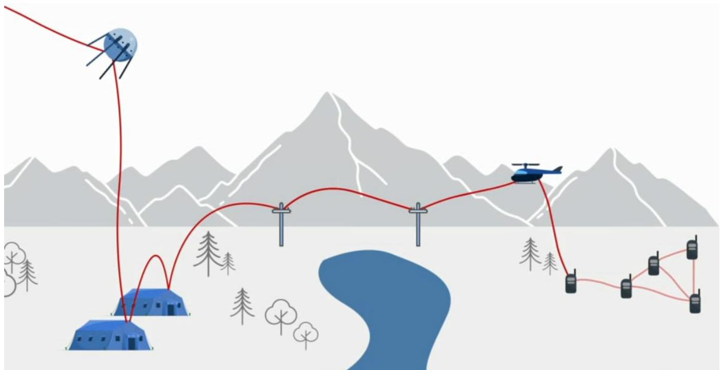
Our WAVESWAY radio system uses the principles of Mobile Ad-hoc Networks (MANET) and allows the creation of self-organizing wireless networks with a dynamic topology.
