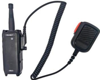
The range in point-to-point mode is up to 3 km for portable stations, 10 km and more for omni-directional repeaters, and up to 50 km for directional repeaters.
